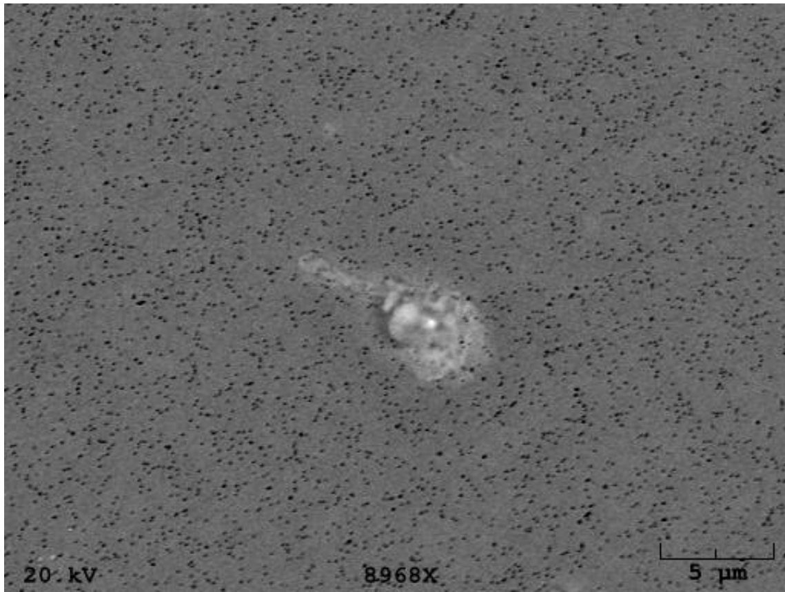
Particle 4-3: Silica Colloid Challenge at 200 Volt Capture and 250 Volt Release
